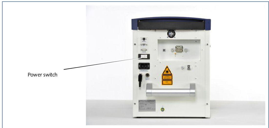
Figure 3: Power switch at the rear panel of the device
