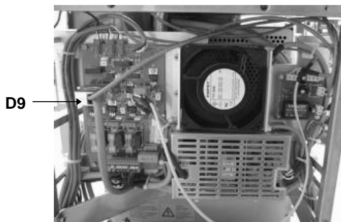
Fig. 25: Connection of service cable to Switching Control PCB → D9 (rear panel of the device)
