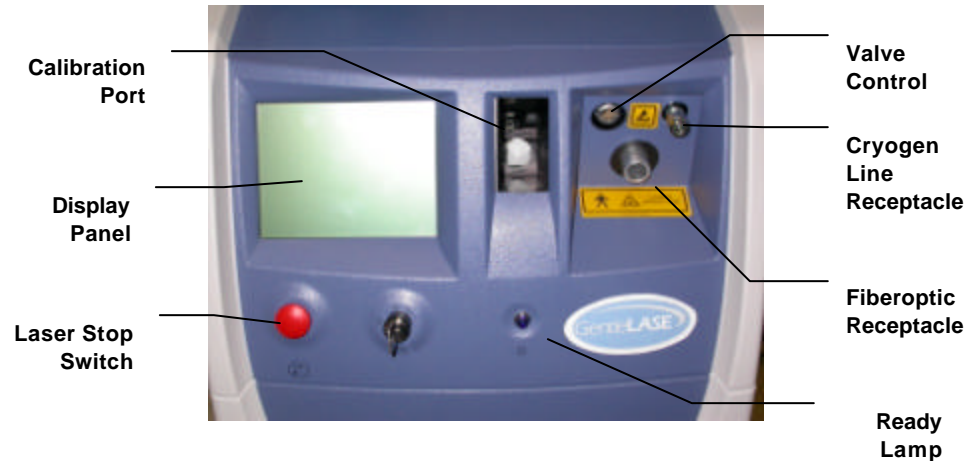
Figure 1 Canister and Delivery System Locations
